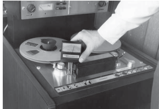
Figure 28-56. Tension measurement. Courtesy Ampex Corp.
