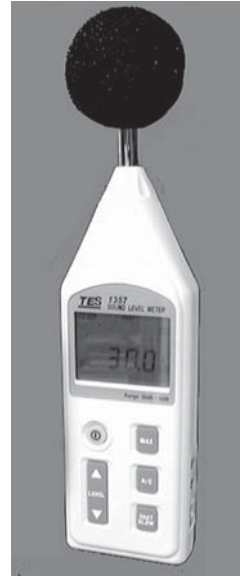
Figure 46-1. A sound level meter is basically a voltmeter that operates in the acoustic domain. Courtesy Galaxy Audio.
