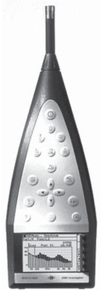
Figure 34-73. Precision integrating sound-level meters and accessory filter sets. Courtesy Brüel & Kjaer Instruments, Inc.
