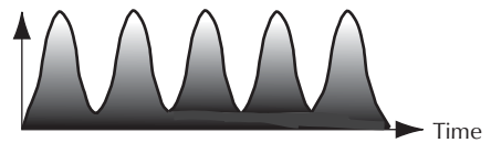
Infrared light with amplitude modulated subcarrier.
