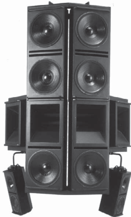
Figure 18-13. Reference Point Array using four 40^\circ \times 40^\circ mid-high enclosures and six low frequency modules in Tri-Polar configuration for vertical pattern control, along with appropriate small full range systems for downfill.
