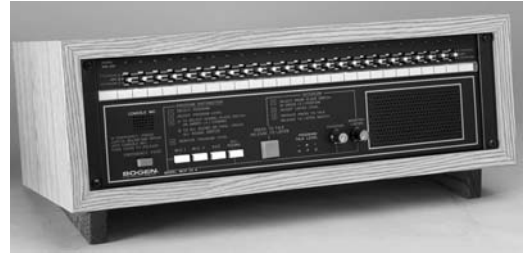
Figure 43-3. Bogen P135A twenty five station intercom. Courtesy Bogen Communications, Inc.
