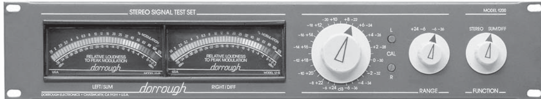
Figure 26-8. Wide range VU meter. Courtesy Dorrough Electronics.
