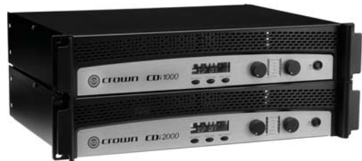
Figure 34-48. A power amplifier with built-in DSP. Courtesy Crown International.
