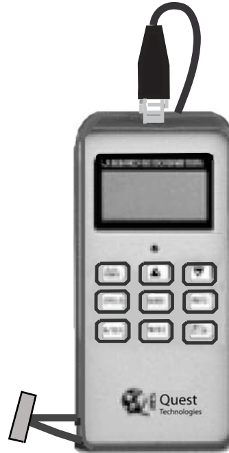
Figure 4-6. Quest Technologies model 300 dosimeter. Courtesy Quest Technologies.
