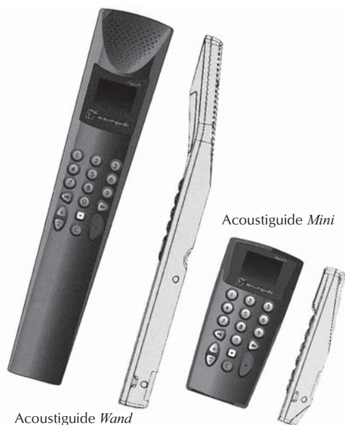
Figure 40-4. Typical wands used in museum systems. Courtesy Acoustiguide Inc.
