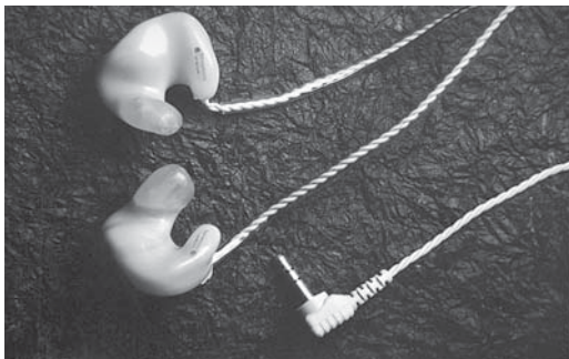
Figure 37-11. Custom molded earphones. Courtesy Sensaphonics.
