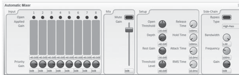
A. Inside a typical Virtual Device from QSC. This shows the sort of controls and indicators found inside the Virtual Devices in Fig. 38-7.
