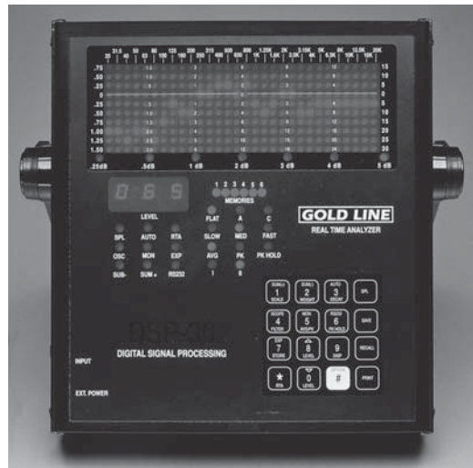
Figure 34-72. A real-time, \frac{1}{3} octave, audio spectrum analyzer. Courtesy Gold Line.
