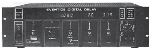
Figure 38-1. Introduced in 1974, the Eventide Clockworks Model 1745M modular digital audio delay was the first to use random access memory (RAM) instead of shift registers for storage of sound. Options included pitch changing and flanging.
