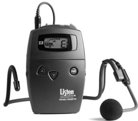
Figure 41-11. Typical high-quality FM transmitter, the Listen LT-700-863. Courtesy Listen Technologies Corporation.
