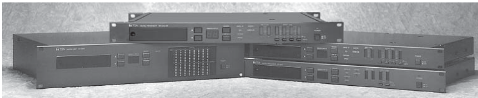
Figure 38-3. TOA Dacsys II digital audio processors (center and right). TOA's second generation digital audio processor (the SAORI was the first), it had a Windows-based control program, which allowed a limited amount of internal reconfiguration of the signal flow. On the lower left is a digitally controlled analog matrix mixer, which could be controlled with the same program.
