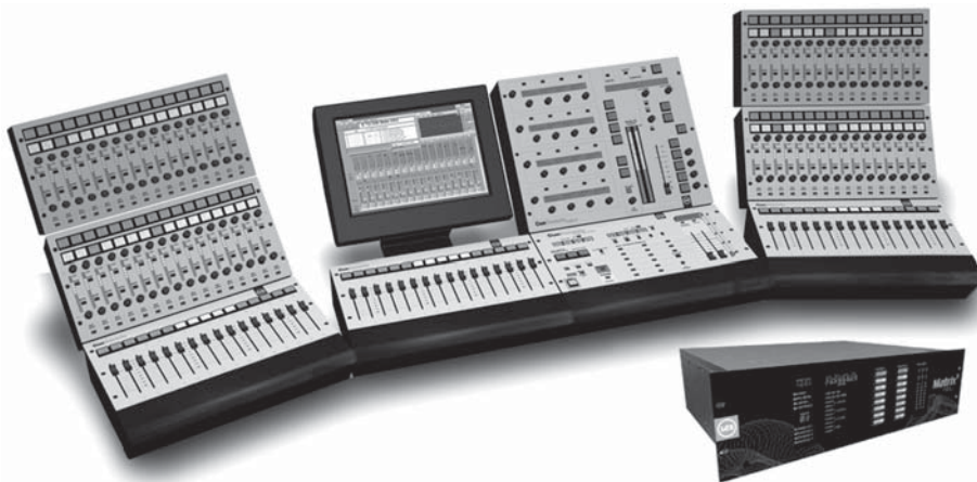
Figure 38-2. The CueConsole from Level Control Systems is a modular audio control surface. The size of the control surface has no direct relationship to the number of audio inputs and outputs controlled. The actual audio processing is performed in Matrix3 processors (lower right corner) located remotely from the control surface. These systems are very popular for Broadway- and Las Vegas-style shows since very large and powerful automated consoles can take up very little of the valuable space in the theater.
