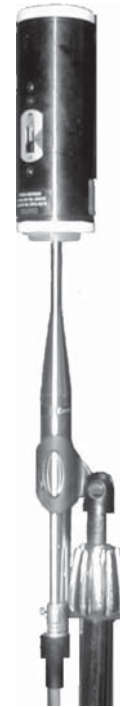
Figure 46-3. A calibrator must be fitted with a disc to provide a snug fit to the microphone. Most microphone manufacturers can provide the disc.
