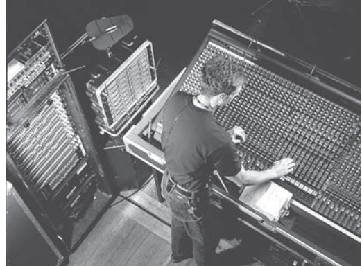
Figure 37-2. Large frame monitor console. Courtesy Shure Incorporated.
