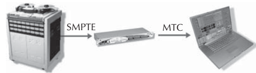
Analog multitrack SMPTE/MIDI interface DAW/sequencer Figure 29-37. SMPTE time code can be easily converted to MTC (and vice versa) for distribution throughout a production system.
