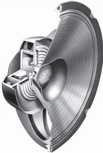
Figure 17-2. Loudspeaker incorporating a whizzer cone.
