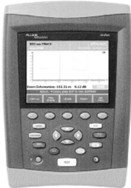
Figure 15-18. OptiFiber Advanced Certifying OTDR. Courtesy of Fluke Networks.
