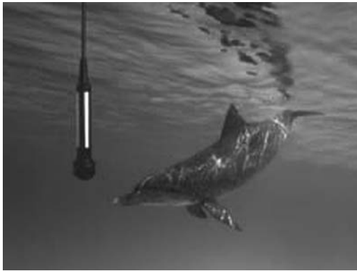
Figure 16-150. DPA 8011 hydrophone. Courtesy DPA Microphones A/S.
