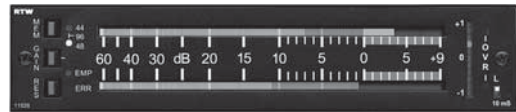
B. RTW 11528G Digital Peak Program Meter + Loudness Meter + Phase Correlation Meter.
