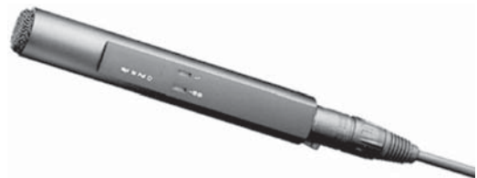
Figure 16-55. Omnidirectional pressure capacitor microphone. Note the lack of rear entry holes in the case. Courtesy Sennheiser Electronic Corporation.
