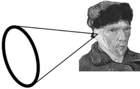
Figure 3-21. Cone of confusion for a spherical head with two holes at the ear positions. If only ITD cues are available, the listener cannot discriminate positions on the surface of the cone of confusion, corresponding to a given ITD . If ILD cues are also available, due to the diffraction of the head, the listener can further limit the confusion range into a circle (the dark “donut” on the figure).
