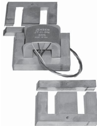
Figure 11-10. Core laminations are stacked and interleaved around bobbin that holds windings.
