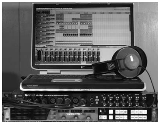
Figure 25-154. A modest-sized DAW running on a USB link between the audio interface unit (center) and the laptop. The (almost free) DAW software allows for 48 simultaneous recorded tracks, with significant audio processing. Complete with shown external mic-amps and computer, the cost of this outfit is about that of a decent microphone; its 1990 equivalent in facilities and performance would have cost the same as a decent car, while the 1970 version would have equated a decent house, which would have been needed to fit it all in, too.
