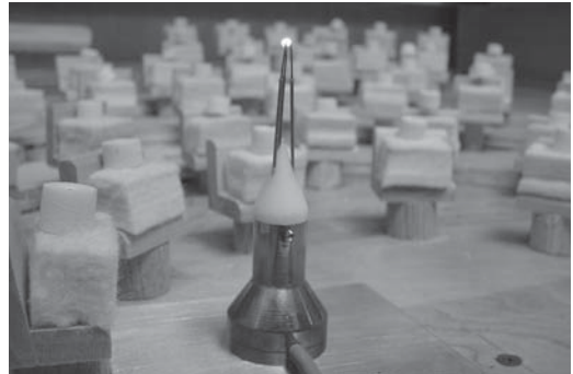
Figure 9-4. A spark generator used in scale physical models. Courtesy Kirkegaard Associates.
