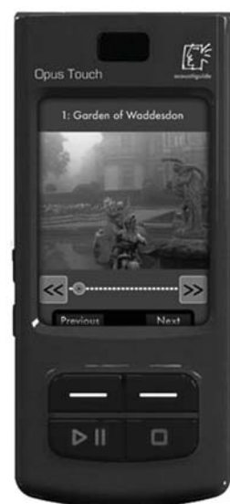
Figure 40-5. Acoustiguide Opus Touch™ screen-based player. Courtesy Acoustiguide Inc.
