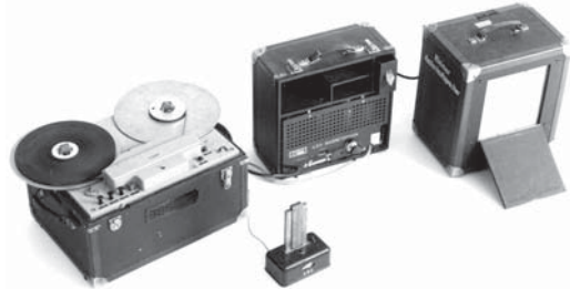
Figure 28-1. German Magnetophon, 1935. This portable magnetophone weighed over 100 pounds. Courtesy BASF Corporate Archives.
