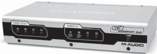
Figure 29-18. M-Audio MIDISPORT 4×4 MIDI interface. Courtesy of M-Audio, a division of Avid Technology, Inc., www.m-audio.com .
